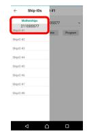
16) To delete a MMSI from the memory of the Rescue Transmitter, tap on the respective number and then tap "Delete".
