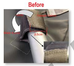
1. Only 2,5cm (length) female Velcro used for bonding.
